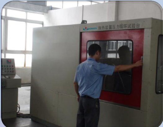
Thermal Cycling Test For life-cycle of radiator
