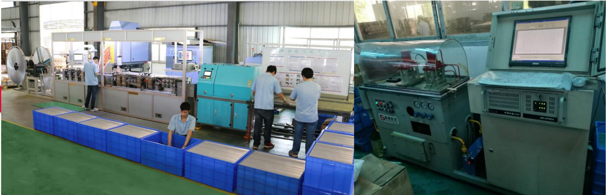
Pressure Explosion Test for tubes
